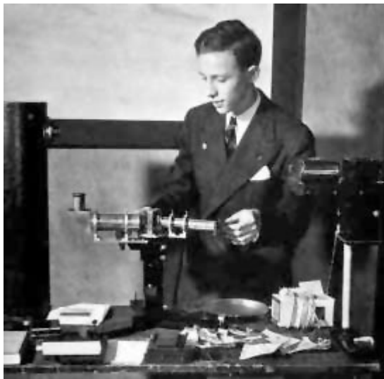
Taken at December 1940 Science Congress talk. At left is a 6 inch richest-field telescope f4, much more portable than my original f8, in the center is the diffraction grating spectroscope, at right a photomicrographic camera, with odd bits of paraphernalia in the foreground.
